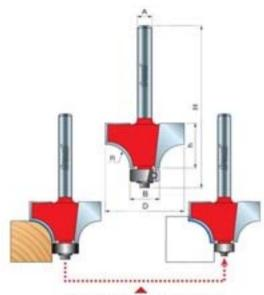
By simply ordering the 3/8" Ball Bearing #62-102 and 3/8" Step Washer #62-311 you will be able to obtain a different profile.
