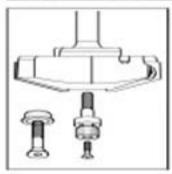
All above Insert Raised panel bits include plug, ball bearing and retaining screw.
