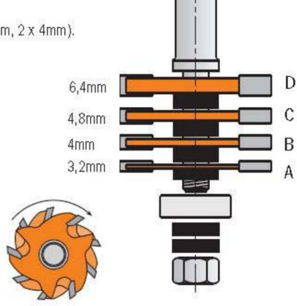
**Note:** the carbide edges of the cutters should never touch; arrange the shims as illustrated below. Use only the thicknesses provided in the set. Be sure all cutters are assembled in the proper rotational direction as shown below. Looking down the arbor the cutters will turn clockwise.
