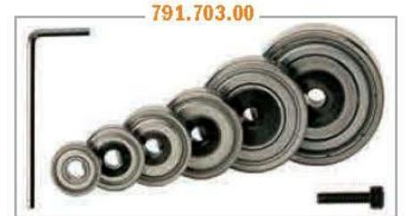
**BE SURE** to keep the black bearing washer right side up to correspond with the bearing rotation when re-assembling the bearing. Improper re-assembly can cause the screw to come loose. Each set comes complete with one rabbeting bit and six interchangeable ball bearing guides.
