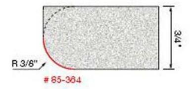
A full bull nose profile can be created by using the above the Under Rounding Bit to create the bottom round over profile and use the Rounding Over Bit (next page) to create the top round over profile.
