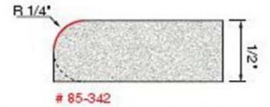
A full built nose profile can be created by using the Under Rounding Bit (previous page) to create the bottom round over profile and use the above Rounding Over Bit to create the top round over profile.
