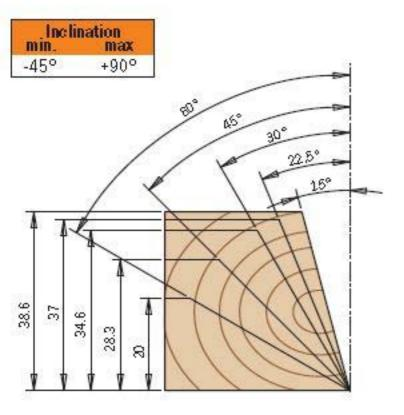
TECHNICAL DETAILS: Tool body in steel, two TC reversible knives in swiveling blade carriers. Cutting on periphery and both sides. Swiveling range towards top 0-45°, toward bottom 0-90°, infinitely variable adjustment according to precise scale. With positive stops at 7,5° through adjustment aide. No displacement of adjusted beveling angle when replacing blades. Righ rotation.
