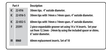
Using standard 30mm or 60mm carbide inserts, this is an easy and inexpensive way to perform trim or rabbet cuts. Please note: spurs are required for all cuts except trimming.
