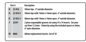
Using standard 30mm or 60mm carbide inserts, this is an easy and inexpensive way to perform trim or rabbet cuts. Please note: spurs are required for all cuts except trimming.
