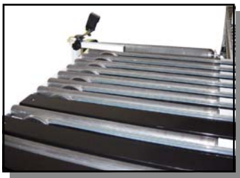
Receiver section showing infed roller and photoeye.
